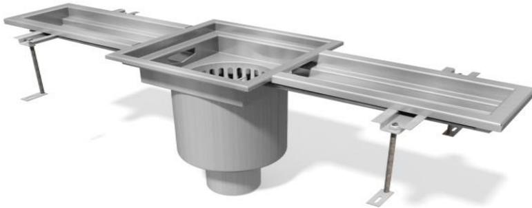
**The sewer KV-170, made of stainless steel 1.4301, provides drainage for the production facilities as well as from the surfaces located outside. The sewer features standard drop of 1.5% and the width of 76mm. Thanks to the fact the bottom of the sewer is V-shaped the amount of standing water is minimized and the hygiene of usage improved. Rims of the sewer are reinforced with flat bars to protect them from damage.**
