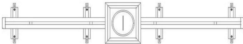
**The slot gutter type KS-60**, made of stainless steel 1.4301, provides drainage for the production facilities as well as from the surfaces located outside. The sewer features standard drop of 1.5% and the width of 20mm. Due to its construction does not require the use of a special cross-section of the cover helps to keep it clean.
