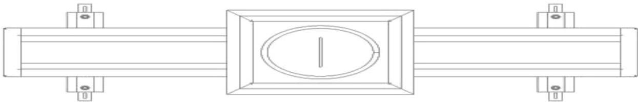
A drain inlet with side or bottom drainage is integrated with the sewer. The sewer features assembly rods allowing it to be steadfastly embedded in the floor, moreover, adjustable mounting shoes allow for positioning of the sewer before laying the floor. The sewer can be manufactured in segments. In order to facilitate transportation and assembly, the segments are provided with screwed flanges. Other sizes and configurations are available upon request.
