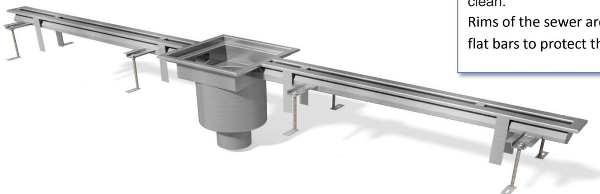
A drain inlet with side or bottom outlet is integrated with the sewer. The sewer features assembly rods allowing it to be steadfastly embedded in the floor, moreover, adjustable mounting shoes allow for positioning of the sewer before laying the floor. The sewer can be manufactured in segments. In order to facilitate transportation and assembly, the segments are provided with screwed flanges. Other sizes and configurations are available upon request.
